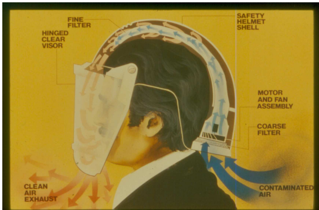
1 2 3 4 5 6 7 8 9 10 11 12 13 14 15 16 17 18 19 20 21 22 23 24 25 26 27 28 29 30 31 32 33 34 35 36 37 38 39 40 41 42 43 44 45 46 47 48 49 50 51 52 53 54 55 56 57 58 59 60 Photograph 5 (b) Diagram of inside the helmet and its workings
