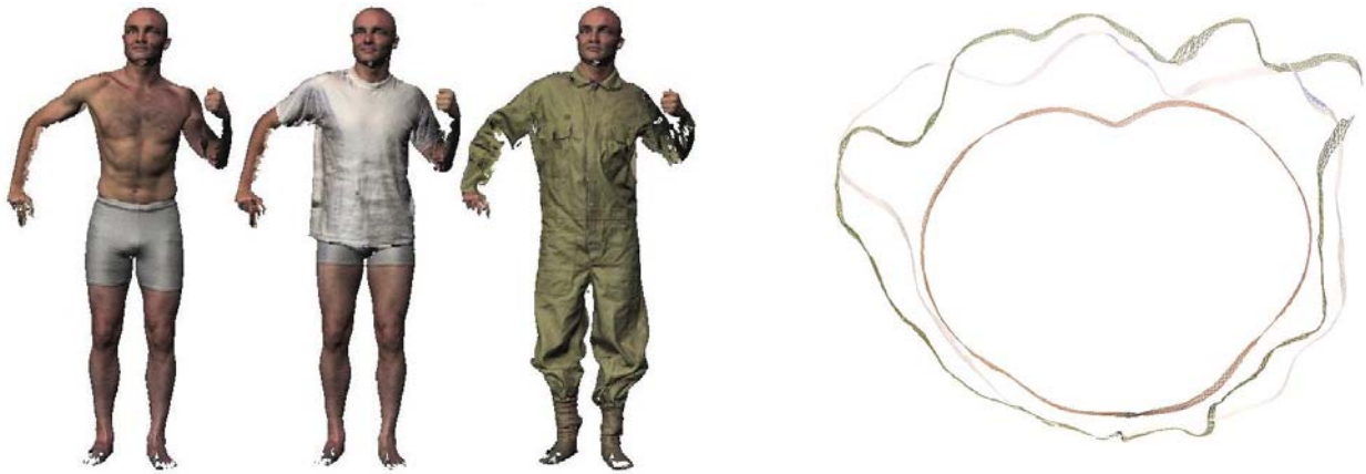
Fig. 2 Frontal and transversal view of the scans for subject 1. The inner object is the torso, the thin line is the T-shirt and the thick line is the coverall. Note that the folds are well covered by the scanner.
