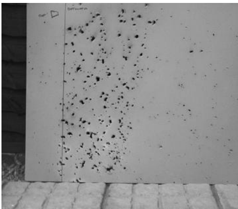
Figure 7: Comparison of fragment distribution on target vertical face. Photograph of the straw board used in the trial (left), and numerical computation (right). Bullet points are used to visualise fragment distribution obtained from the model.
