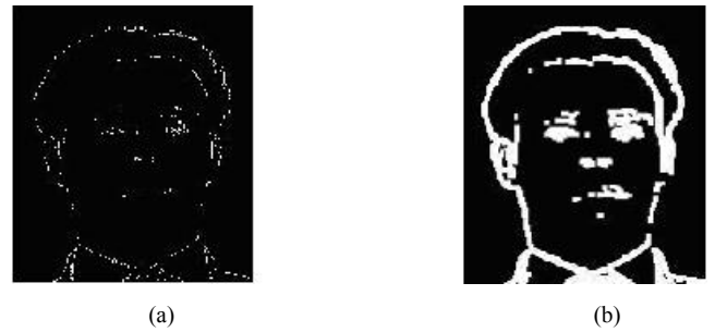
Figure 5 Morphological Dilation (a) Image Before Dilation (b) Image After Dilation
