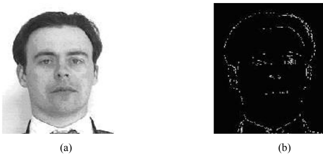
Figure 4 Edge Detection (a) Grey Level Image (b) Detected Edges
