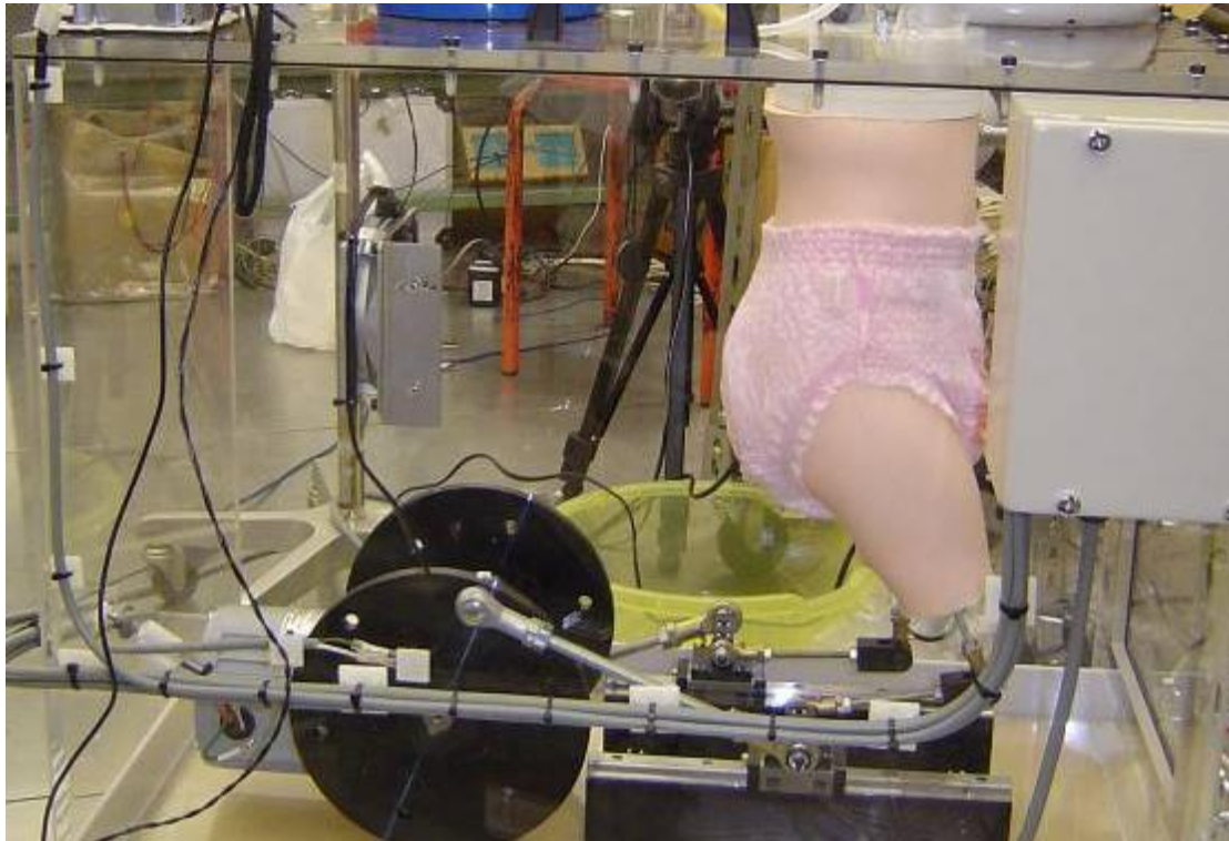
Fig.3 Photograph of the ventilation apparatus showing the manikin model and the movement mechanism inside the Perspex box. The box walls facing the front and back of the manikin are open to the environment to avoid CO 2 buildup.
