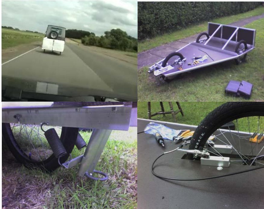
Figure 3: The trailer through driver's view in the track (top left), during development (top right) and details of the auto-brake mechanism (bottom left/right)
