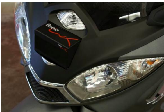
Figure 5: Integration of the Ibeo Lux Laserscanner
