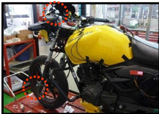
Figure 19: Anti-dive suspension on the TVS motorcycle
