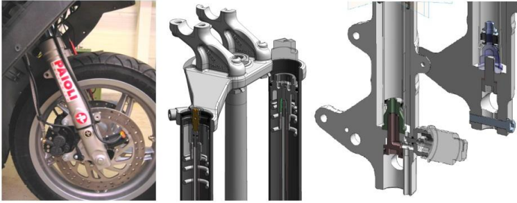
Figure 13: Semi-active front fork installed on the Malaguti
