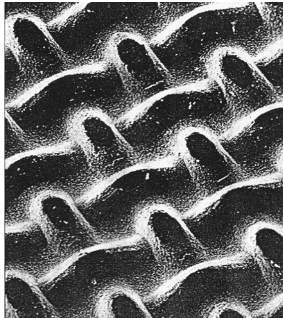
Figure 4: Surface features of a 0.2 µm rated Ceramesh membrane.
