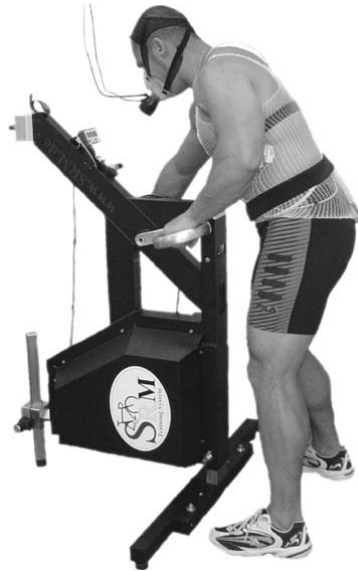
Fig. 1 Image of the modified SRM arm ergometer used for America's Cup grinding performance analysis. Crank length was 0.25 m and the distance between the handles was 0.44 m.
