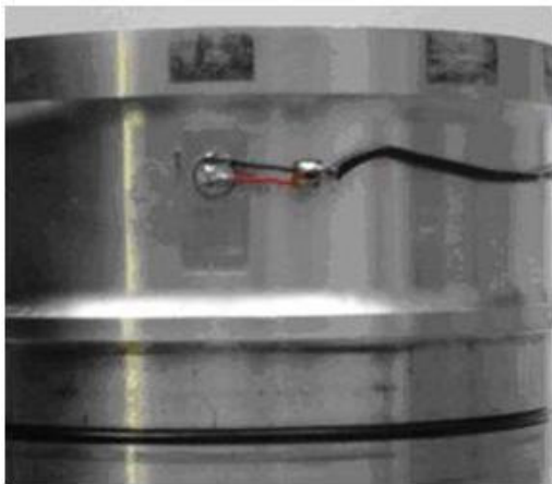
Figure 2: Photograph of the cylinder liner with the ultrasonic transducer bonded to the wet side.
