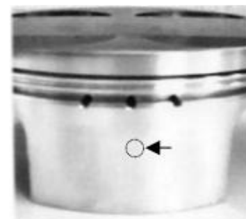
Figure 9a: Area where average film measured on the piston skirt indicated by the circle
