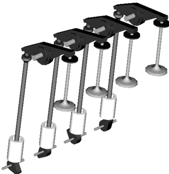
Fig. 1 Schematic representation of a valvetrain system for a four-cylinder in-line engine
