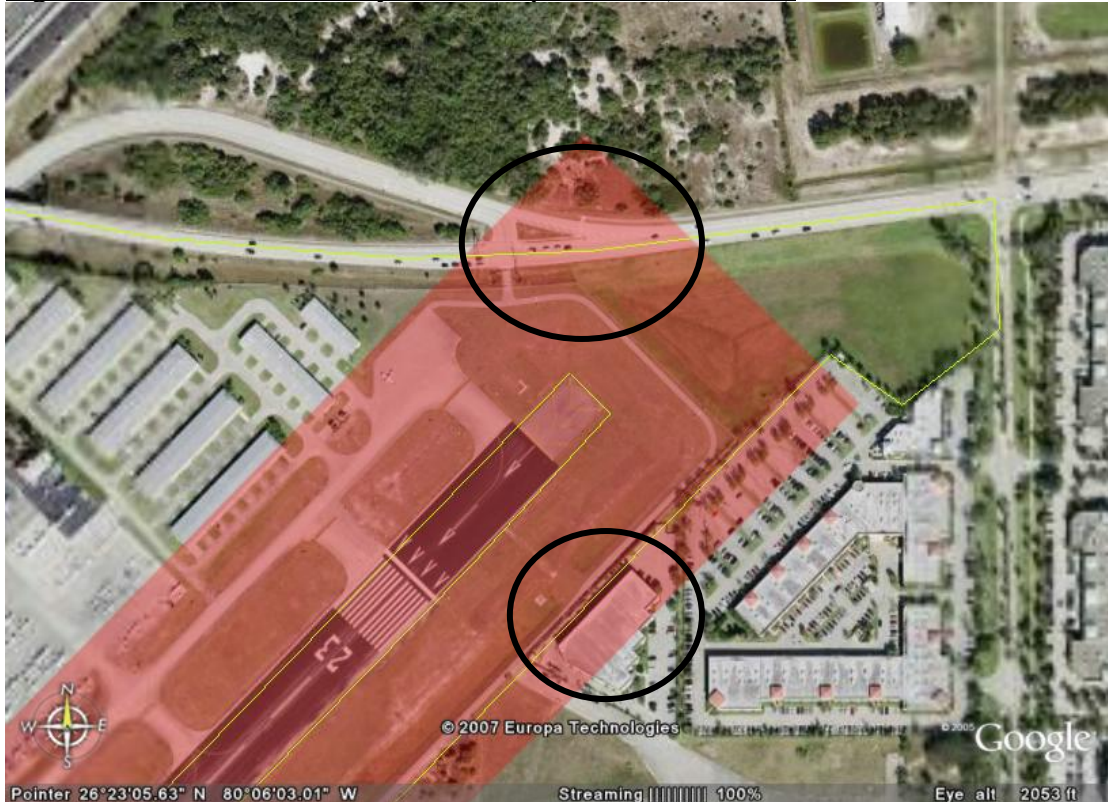
Figure 20 BCT end of runway 5 ASA requirement (TLS 10^{-7} )
