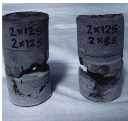
Figure 8. Example of voidage behind reinforcement (photograph)
