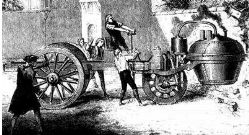
Figure 1: The first vehicle (“fardier à vapeur” Cugnot 1770) and the first known vehicle accident
