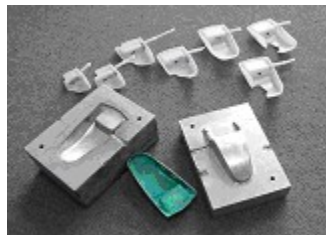
Fig. 12. Metal spraying, TUCN
