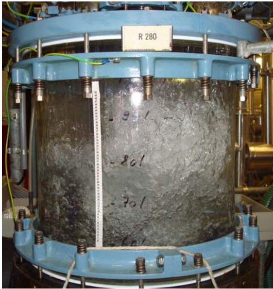
Figure 1 Swelled liquid in a 100 L pilot plant vessel.
