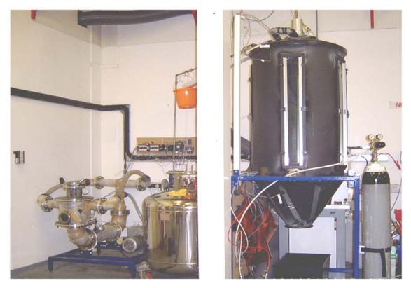
Figure 2. The spray-freeze-drying apparatus used at Loughborough. Spray-freezing initially occurs in the large (black) chamber located on the right of the photo. The spray frozen particles are collected from the base of this chamber and transferred to the sub-atmospheric fluidized bed freeze-drying apparatus on the left of the photo.
