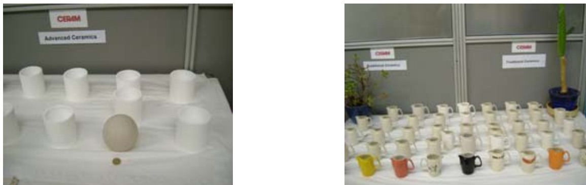
Fig. 3: Hollow ceramic items produced by the ICRM route.
