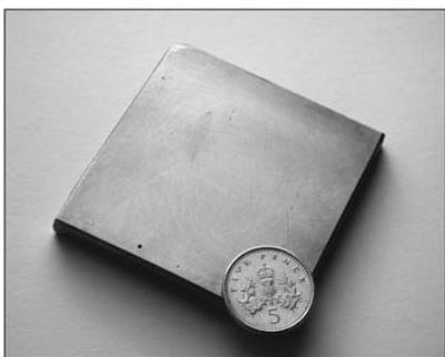
4 Macro photograph of Sodium Hydride cleaned nickel tooling plate (after water jet washing & drying). Water contact angle of 32° measured
