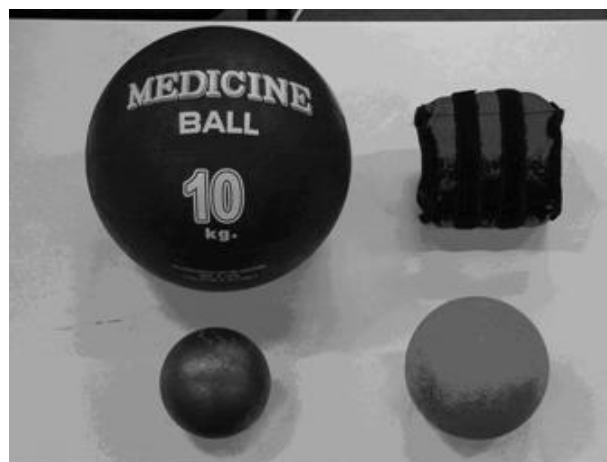
Figure 1. Objects used to assess the impact attenuation of the rugby pad. From top left, clockwise: medicine ball, weight belt, indoor shot and outdoor shot.
