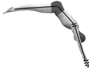
Figure 2. The four segment gymnast - high bar simulation model with damped springs representing bar and shoulder elasticity.
