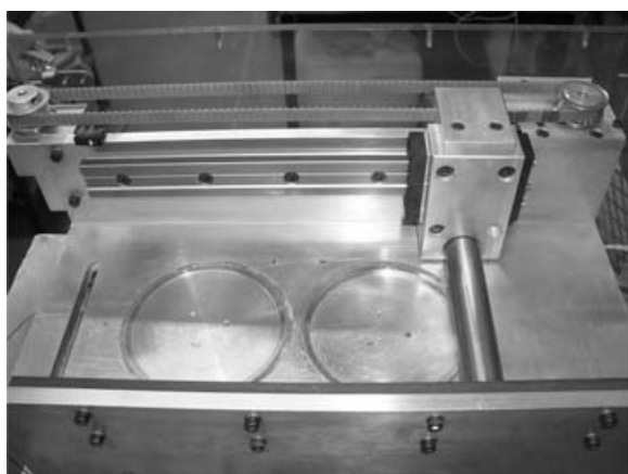
Fig. 1 Photograph of the experimental chamber showing the build and feed cylinders and feed mechanism
