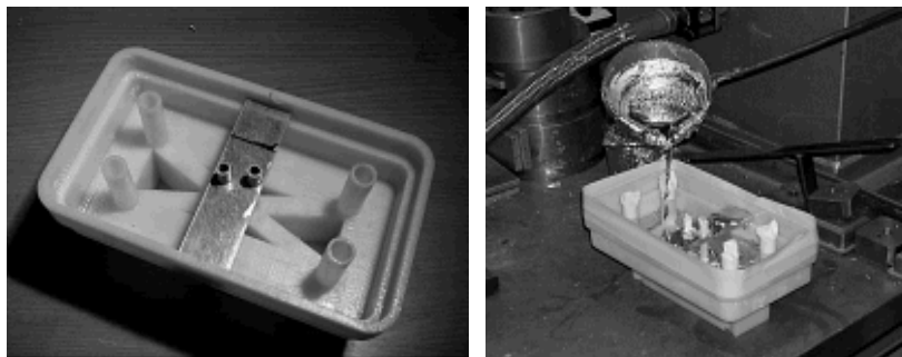
Figure 6 SL shell (left) and backfilling process
