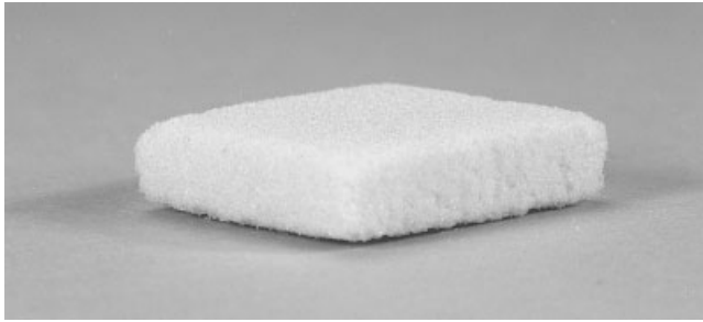
Fig. 3 A 30-layer 'green part'. 15 mm × 15 mm × 3.8 mm
