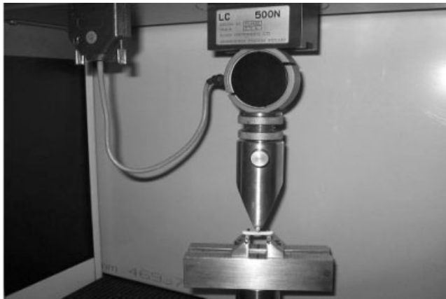
Fig. 9 Three-point bend test
