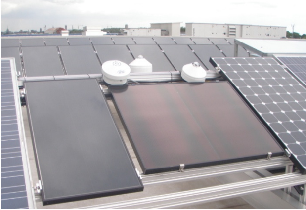
Figure 4: Sensors measuring horizontal and plane-of-array irradiance and spectral distribution.
