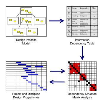
Figure 3 The Analytical Design Planning Technique (ADePT)
