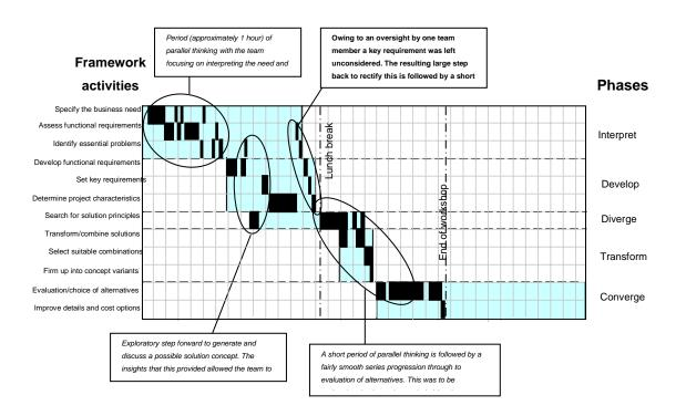
Figure 2 Example of design phase progression (MDP project)
