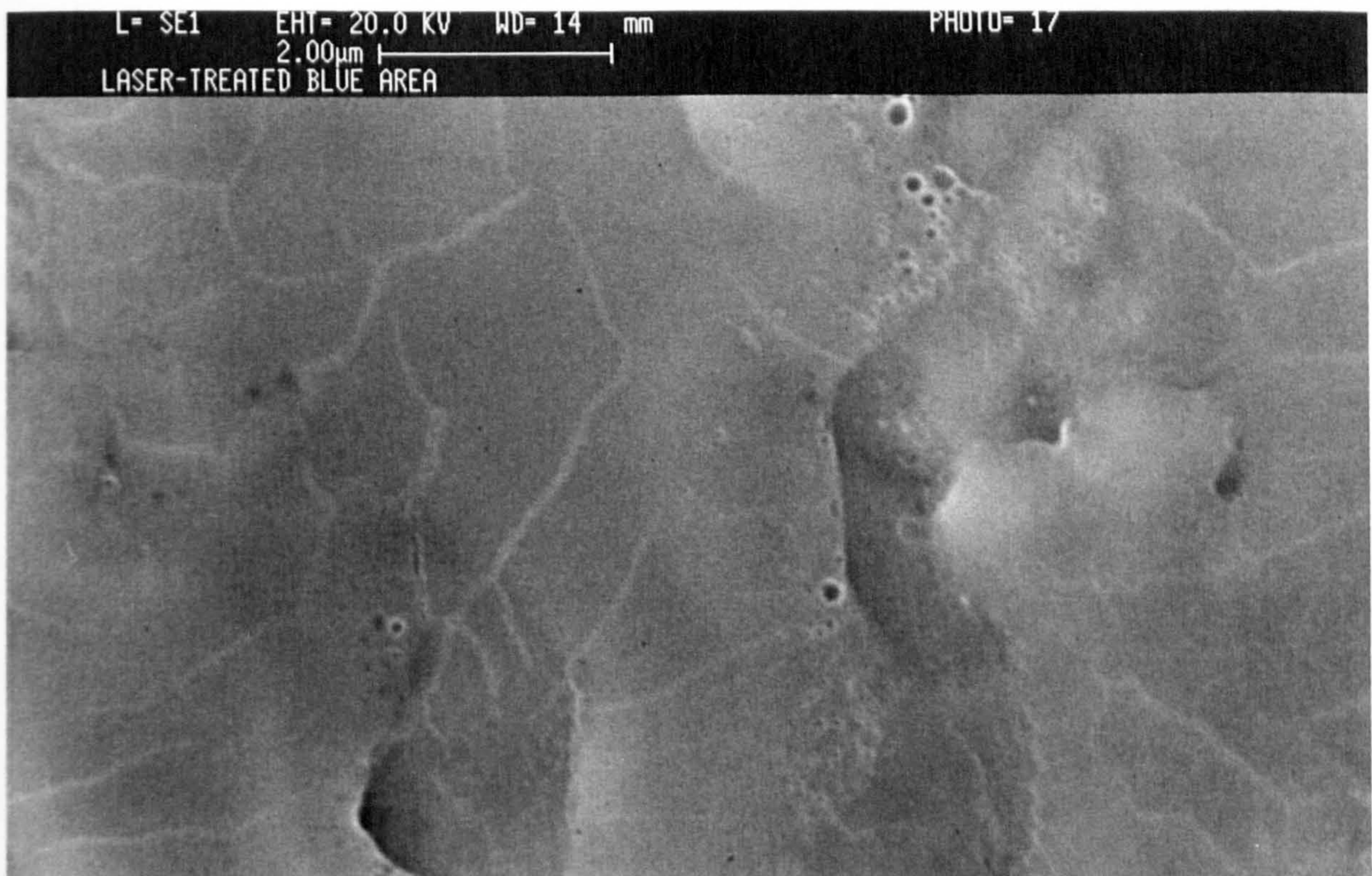
Figure 11 - SEM Micrograph from a CO 2 -laser Treated CR1 Mild Steel Sample, Dark Blue in Colour, at 13000 Magnification.
