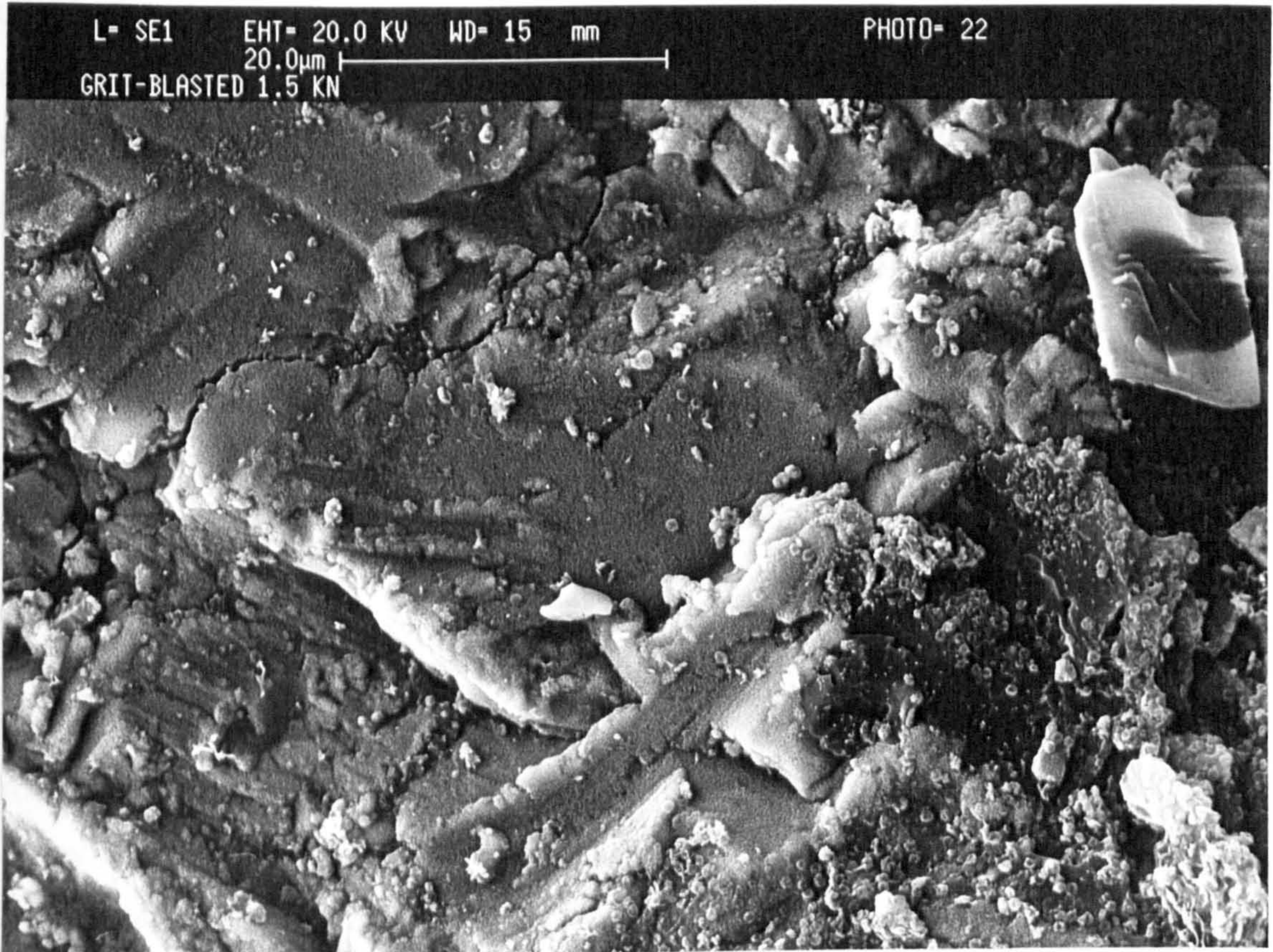
Figure 30 - SEM Micrographs to Show a. the Metal, and b. the Adhesive Sides of a Joint Prepared with Grit-blasted Adherends Following SSLS Testing at a Load of 1.5 kN and Simultaneous Immersion in DI Water at 60°C.
