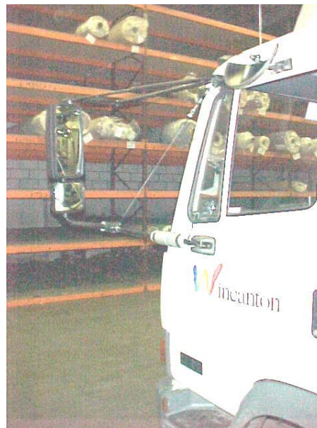
Figure 2. Modified Leyland/Daf FA45 - near-side mirrors
