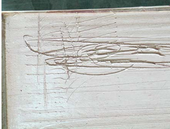
Figure 13: The tiles before the fire, with lines inscribed in the porcelain, metal colour oxides painted to fill the lines, and after being cleaned with a sponge, a technique derived from graphic copper etching.
