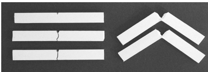
3 Notched Charpy sample with two examples of breaks and 'non-breaks'
