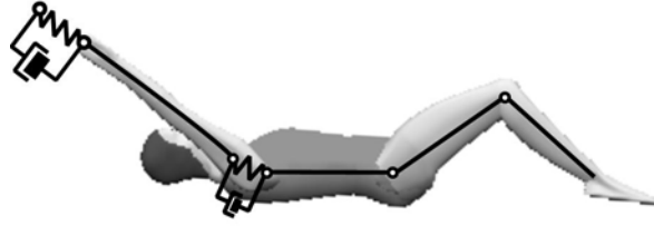
Figure 2. The four segment gymnast / high bar simulation model with damped springs representing bar and shoulder elasticity.
