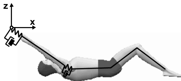
Figure 3. The four segment gymnast – high bar simulation model with damped springs representing bar and shoulder elasticity.
