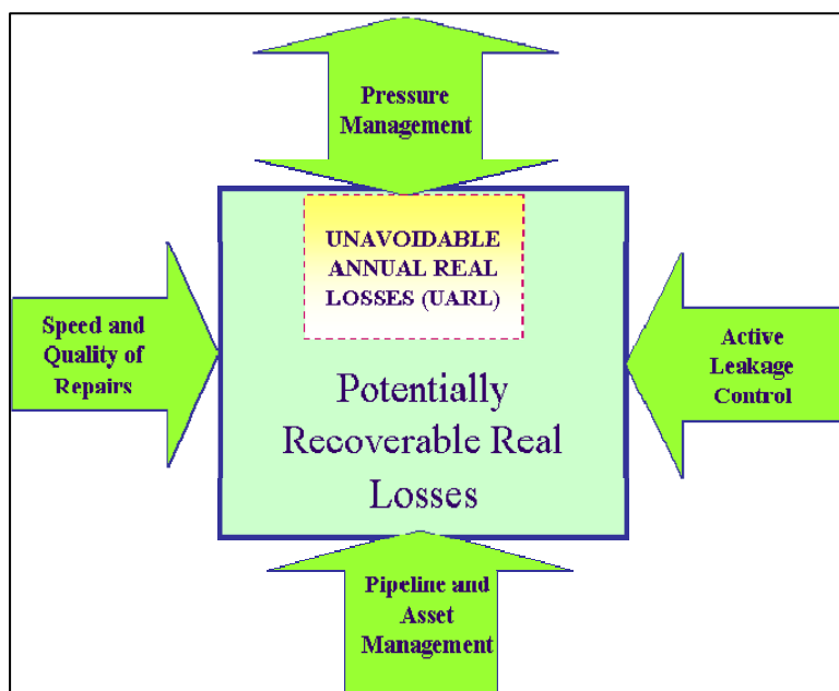
Figure6: Components of water loss management strategy, as developed by IWA (Source: Liemberger and Farley, 2004)
