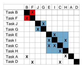
Figure 4. Example of DSM Analysis before and after partitioning
