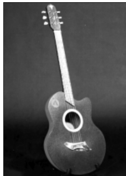
Figure 9: P1 - The first prototype polymer guitar (with a wooden neck).
