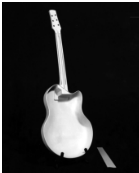
Figure 5: RIM polyurethane back and fingerboard acoustic guitar mouldings.
