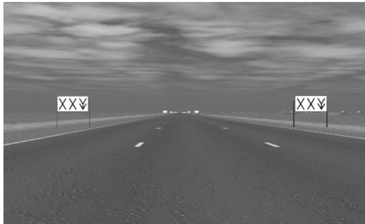
Figure 2: Screen shot from the LCT. In this instance the driver has to change from the centre lane to the right lane.
