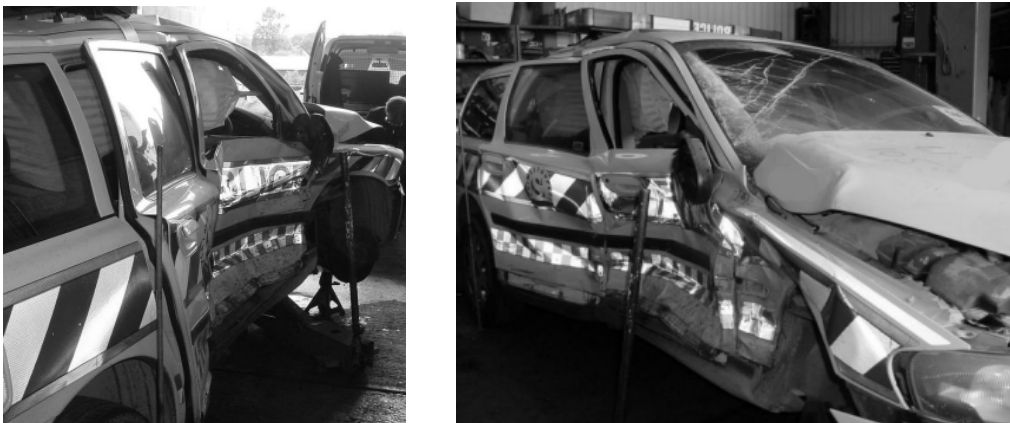
Figures 1 & 2. Case 1 - side impact damage
