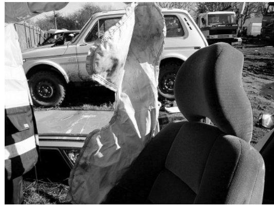
Figures 6 & 7. Case 2 - Intrusion and deployed side airbags at driver's position
