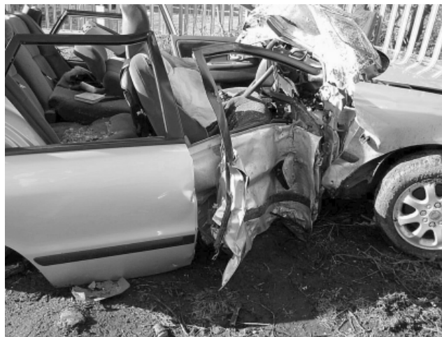
Figure 5. Case 2 - Side impact damage
