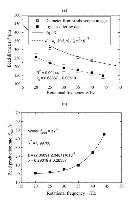
Figure 9. The characteristics of the bead formation: (a) diameters of hardened beads measured by light scattering compared to the diameters of the ejected drops observed on stroboscopic images. (b) bead production rates at different rotational frequencies.
