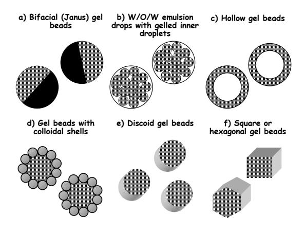
Figure 2. Examples of complex hydrogel microbeads fabricated through various microfluidic and membrane emulsification routes.
