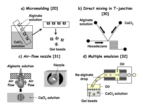
Figure 3. Microengineering techniques for production of calcium alginate microbeads by ionotropic gelation. The techniques are applicable for production of hydrogel beads of any biopolymer.
