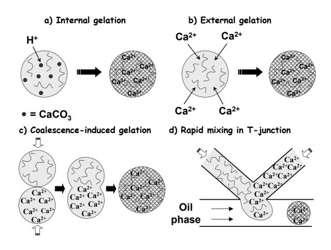
Figure 4. Main strategies for production of hydrogel beads by ionotropic gelation. For gelation of positively charged biopolymers, multivalent anions must be used instead of Ca<sup>2+</sup>.
