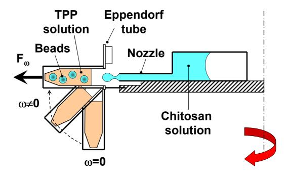
Figure 6. Schematic of the experimental setup consisting of centrifugal platform with a polymeric micronozzle and Eppendorf tube in a swinging bucket.
