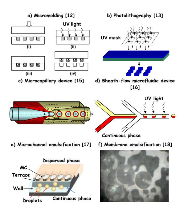
Figure 1. Innovative microengineering techniques for fabrication of hydrogel microbeads.
