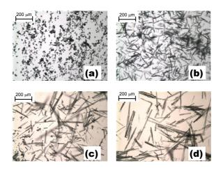
Fig. 11. Microscopic images of seed (a) and product crystals for the three operating modes: (b) coolingonly; (c) antisolvent-only, and (d) combined.
