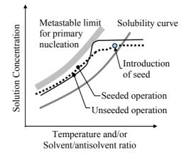
Fig. 1. Operations of seeded and unseeded batch cooling and/or antisolvent crystallizers.
