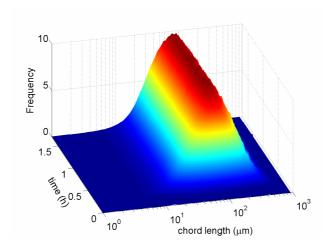
Fig. 13. FBRM CLD for the antisolvent system.
