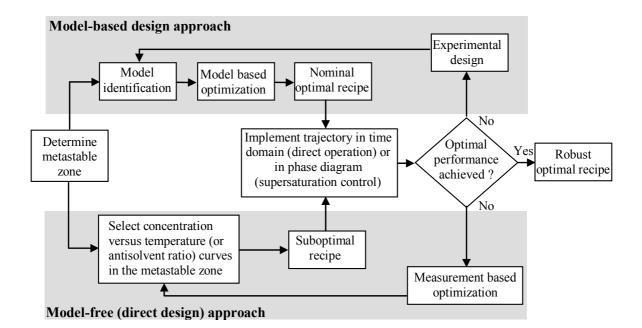
Fig. 2. Schematic representation of the model-based and model-free (direct design) approaches for
