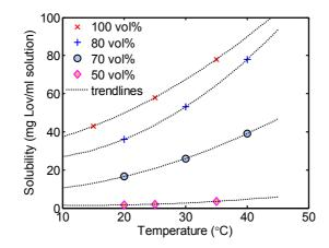
Fig. 4. Solubility curves of lovastatin at different acetone concentrations.
