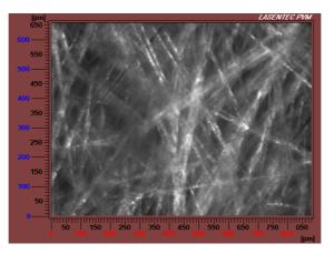
Fig. 16. PVM image of lovastatin crystals.
