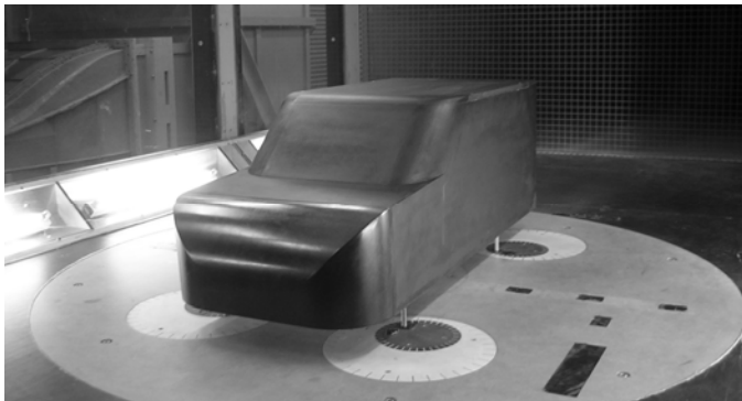
Figure 1 2-box model installed in the Loughborough tunnel
