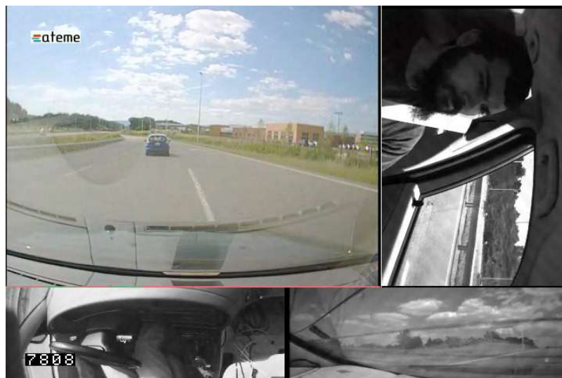
Figure 2.2 The four video camera views in the large-scale SHRP2 study (Source: www.trb.org )
