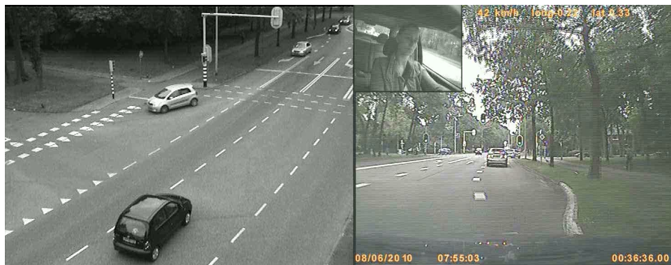
Figure 3.7 Video image from one of the site-based cameras (left) and from the equipped car (right)
