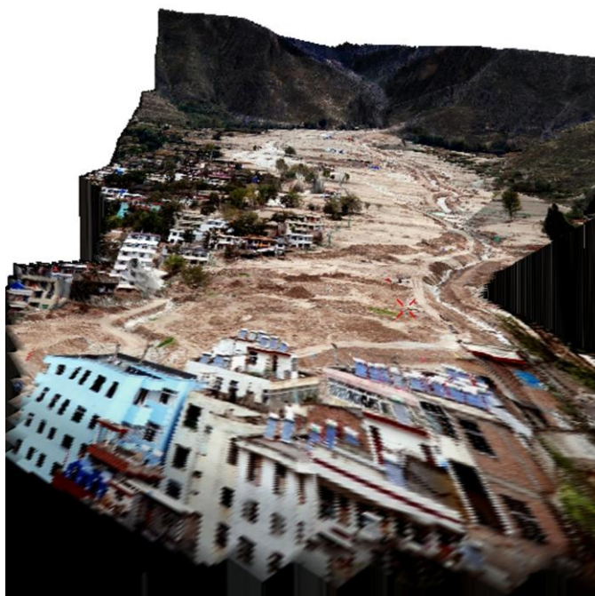
Figure 3. DEM/orthophotograph of the lower depositional environment in Zhouqu after the landslide event
