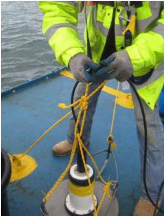
Figure 5.11 Geophone sledge deployment.
