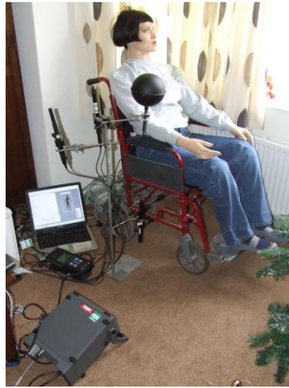
Figure 3: Heated thermal manikin 'Victoria' being used at the test house for thermal comfort trials
