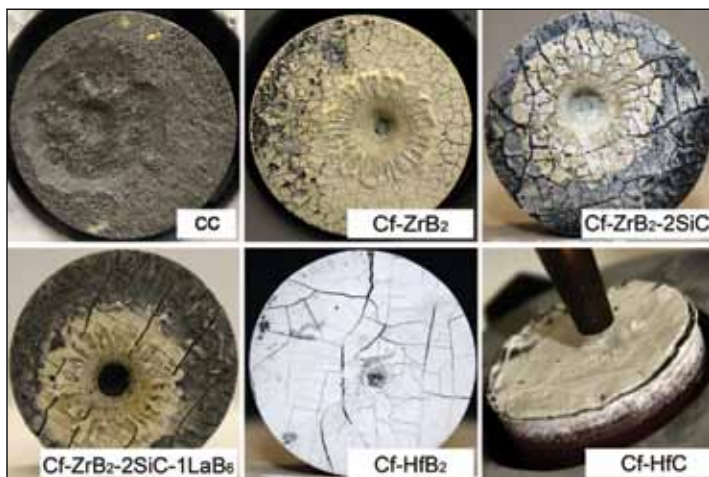
Figure 13 Comparison of carbon-carbon (CC) and carbon-fiber (Cf-) UHTC composites after 60 seconds oxyacetylene testing. Diameter of the composites was 30 millimeters.
