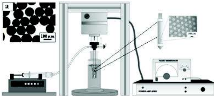
Fig. 1 Image of produced droplets for condition f=70 Hz, A=0.4 mm corresponding to the maximal shear stress of 3 Pa, oscillating membrane system, tubular membrane and surface of used membrane.
