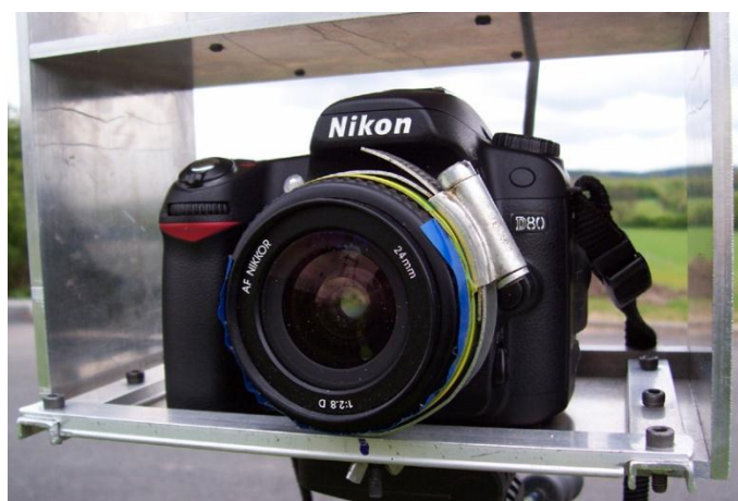
Figure 3.10: Modified approach of camera fixture: hose clip.
