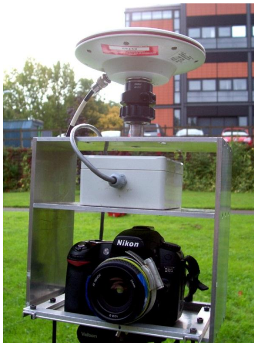
Figure 3.8: Recording system mounting frame with camera, orientation sensor, and DGPS antenna.
