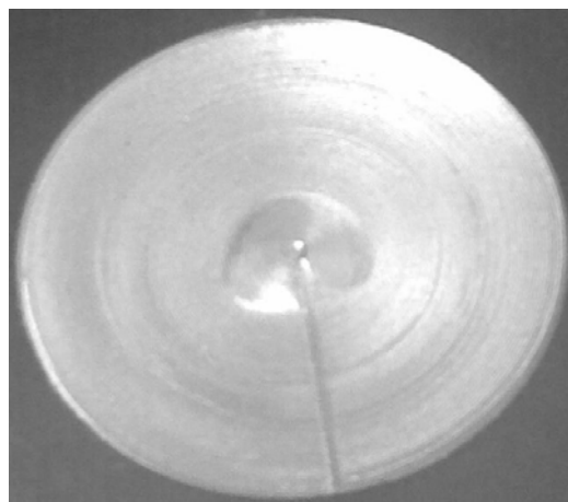
Figure 4: Machine damage to a circular indentation
