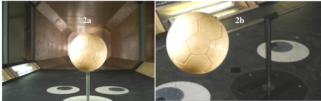
Figure 2a Below Mount; 2b Rear Mount of a ball in the wind tunnel.
