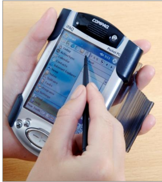
Fig. 1 Interacting with a PDA using both power and pinch grips
